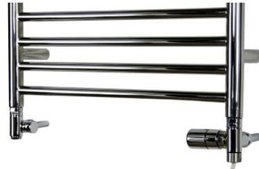
This eliminates the need for a T-Piece, keeping the pipe centres symmetrical and this combination allows you have control over the central heating but does not allow you to have control over the electric element. These valves do not protrude outside the rails dimensions. The Standard Element has a factory fitted thermostat but this is not adjustable.
