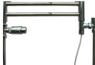
This combination allows you to have control when the central heating is on but does not allow you to have any control over the element (the Standard Dual Fuel Kit has a factory fitted thermostat but this is not adjustable). The lockshield valve does not fit under the bottom bar so has to go on the outside of the rail.
